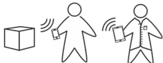
Figure 2. Marionette setup of the ubicomp interaction. For the user, the information seems to be coming from the object, whereas in reality, the researcher sends this information to the user's device.
