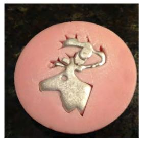
Figure 5: Final mold poured with pewter.
