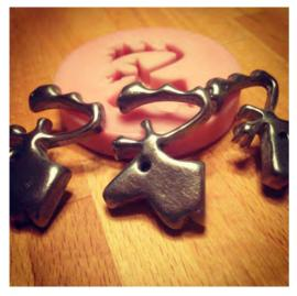
Figure 1: Pewter reindeers casted in a silicone mold.
