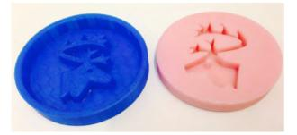
Figure 4: 3D printed intermediary mold (left) and final silicone mold (right).
