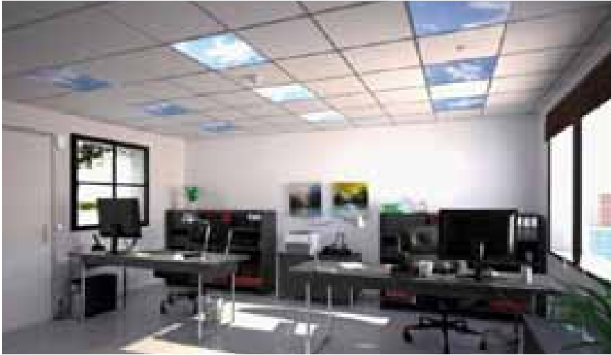
Figure 1: The vision of a daylight office, as the company shows it in its sales brochure. An office environment with skylight illuminaires in the ceiling and an artificial window in the darker corner.
