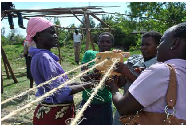
Figure 5: The first Rope Making machine tested in Dunga with sisal fibre, October 2013. Photo: Helena Hansson
