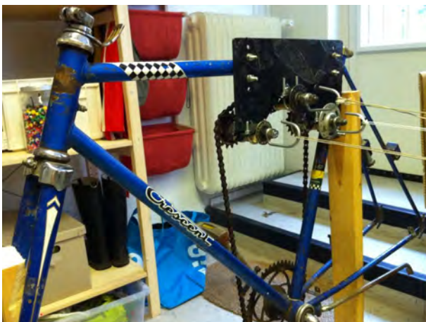
Figure 3 The second rope-making machine made out of pieces from re-cycled bicycles, Gothenburg 2013. Photo: Helena Hansson
