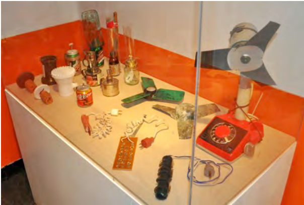
Figure 1: Some examples of various objects engineered from rationed items in Cuba, from kerosene lamps from jars and cans to fans made from records and rotary phones. Credit: Ernesto Oroza from exhibit “Technological Disobedience” at the Miami Science Museum 2014.
