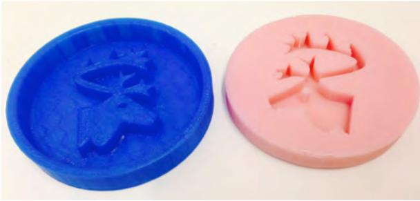
Figure 4: 3D printed intermediary mold (left) and final silicone mold (right).
