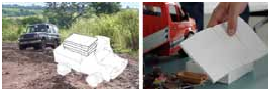
Figure 1. The combo concept. All components of the sustainable energy generator packed in one box to be transported by truck. Sketches and models are based on viewing video footage.
